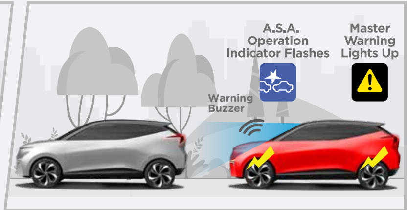
Warning buzzer + primary brake (weak)
