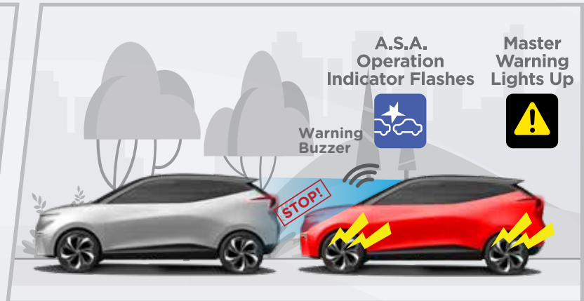
Warning buzzer + secondary brake (strong)
